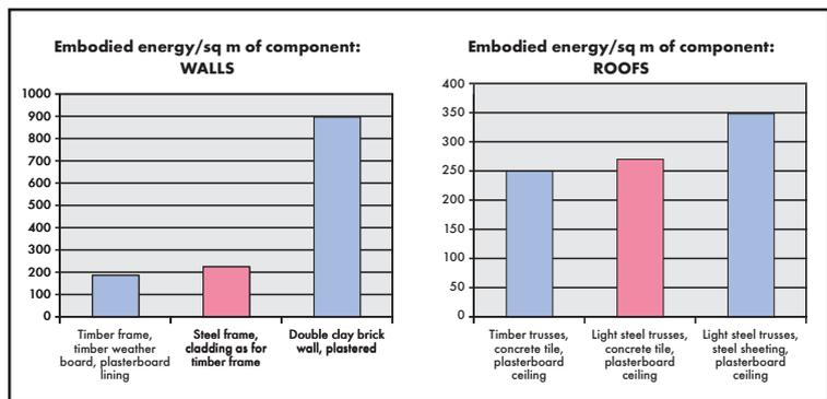
Graph 1: Embodied energy per assembly of materials, per unit area.
